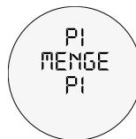
During pre-brewing, the coffee grounds in the group handle are moistened before the actual extraction. You can set the duration of the pre-infusion in 5 levels. You can switch off the pre-infusion with level P 0.
