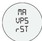
Resets the pressure profile setting for the selected user for the manual preparation via the hand lever to the factory settings.
