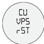
Resets the pressure profile settings for the selected user for the ☕ & ☕ buttons to the factory settings.
