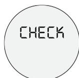
This means that the rotary knob for steam or hot water is not properly closed.
