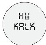
This is the descaling programme for the hot water circuit.
