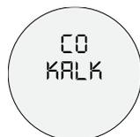
This is the descaling programme for the brewing circuit.
