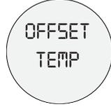
You can adjust any deviations in the brewing temperature here. The temperature can be set in the range from -10 °C to + 10 °C in 1 °C increments. The default setting is 0. Text is displayed continuously.
