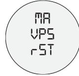
Resets the pressure profile setting for the selected user for the manual preparation via the hand lever to the factory settings.
