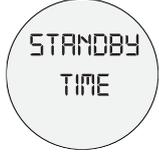
The time until automatic switch-off can be set. Can be set from OFF to 5 - 60 min. in 5 minute intervals. The default setting is 30 minutes. Text is displayed continuously.
