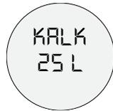
Here you can set the flow rate until the next descaling. You can select between 12 l, 25 l and 50 l.
