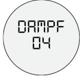
This shows the setting for the steam. You can select whether the steam shall be wet or dry. You can select between 7 stages.
